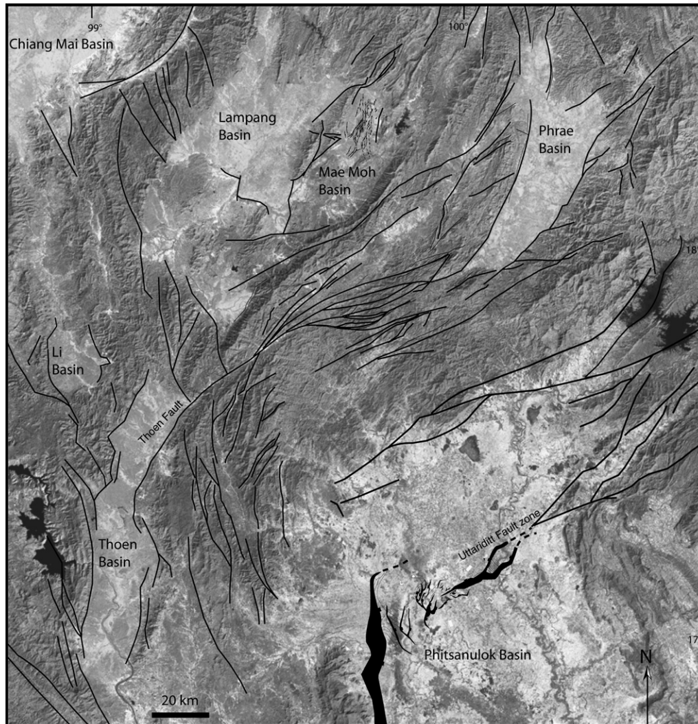
Fig. 12. Fault and basin map of south Northern Thailand illustrating a mixture of Cenozoic fault orientations, the NNE–ENE–WSW trends are interpreted to follow zones of weakness in pre-Cenozoic rocks, NE–SW to ENE–WSW fabrics related to the Indosinian orogeny are particularly prominent in the region (see Fig. 2 for location).
