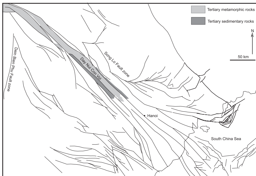
Fig. 18. Map of Cenozoic faults that could be transferring displacement away from the main Red River Fault zone trend passing from onshore to offshore, Vietnam. Fault patterns based on Leloup et al. (2001) (onshore), Rangin et al. (1995) (offshore) and satellite interpretation. The many fault strands and splaying pattern suggest that a considerable amount of the Red River Fault zone displacement may be lost around the onshore/offshore transition.
